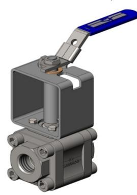
A locking lever handle is standard on the entire 35 Series. The -LXH extension option provides customers with the added benefit of adding a minimum of 3" to elevate the locking handle above the piping, ensuring adequate clearance for insulation and other obstructions and ease of operation.
