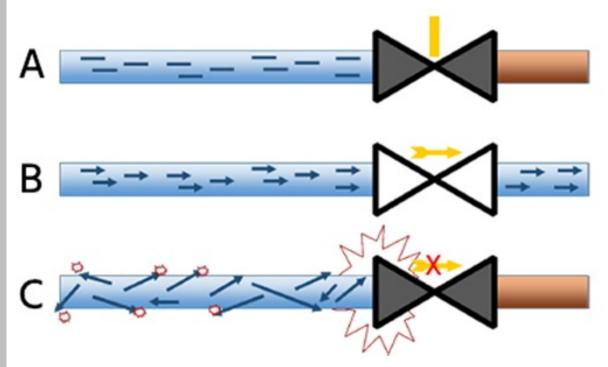
For the sake of this example, also consider the time required to close each of these valves. The ball valve can be closed in a second, while the gate valve takes about 8 seconds. Upstream pipe length is also a consideration, so let's use about 100 ft.
